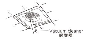
Wipe the dust off the fan body with a soft cloth moistened with kitchen detergent, and then clear it with a clean soft cloth.
