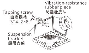
② Install the fan body on the anchor bolt refer to the following form. (M8-M10, not supply)
