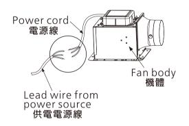
⑥ Make the power cord pass through the wooden frame, push the fan body into wooden frame, to fix the fan body and adaptor assembly.
